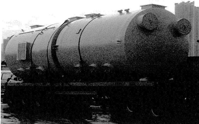
Two dual bed construction filter houses on a 12m length trailer delivered to site
